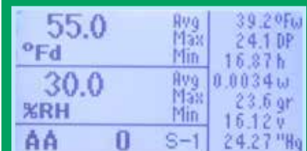
Humidity screen display 2 Humidity results are automatically adjusted for local air density.
