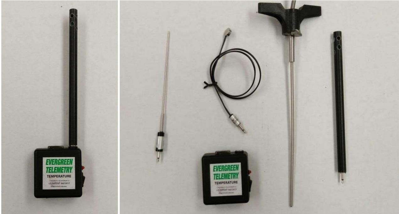
Temperature Sensors (S-T-x) are comprised of a (2x2" x 1/2") Radio Module and a Probe (PR-T-x). Radio Modules and Probes can be purchased together or separately. Any Temperature Probe can be inserted into any Radio Module; the resulting Temperature Sensor will still meet the specs.
