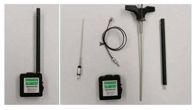
Temperature Sensors (S-T-x) are comprised of a (2x2" x ½") Radio Module and a Probe (PR-T-x).
