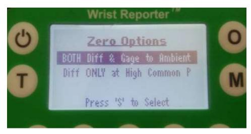
**Method Two—Zero to Lo Port Pressure.** This procedure is for applications like balancing valves when the Gage / Common pressures are relatively high, and the Differential pressure is low. For instance, Gage Hi = 80 PSI; Gage Lo = 79 PSI; Diff = 1 PSI = 2.3 ftwc. This procedure zeroes the Differential Sensor while leaving the Gage Sensor unchanged and therefore able to display accurate Gage results.
