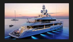
Project Orion is the third in Heesen's advanced 50-metre FDHF aluminium series with hybrid propulsion.
