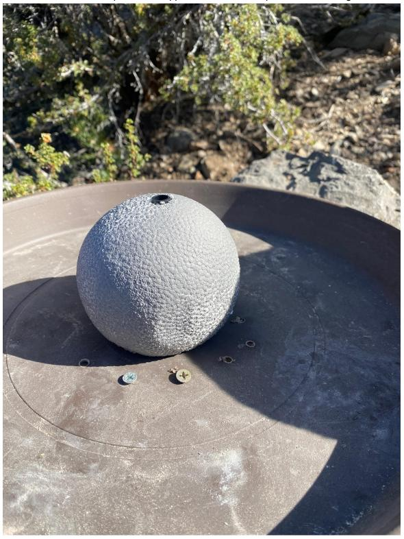
Ball is secured with two screws and holes drilled in plastic tray near ball for a return to the bucket. Holes are plugged with screws to maintain water level and removed if more return flow is required.
