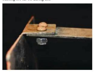
6. Drill a hole in the opposite end of the metal bar and secure it to the remaining PVC cap with a nut and bolt.
