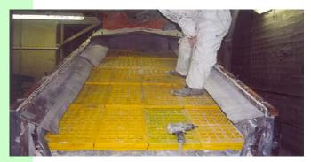
A range of polyurethane screen panels are available which can be fitted onto "step"type screen frames.
