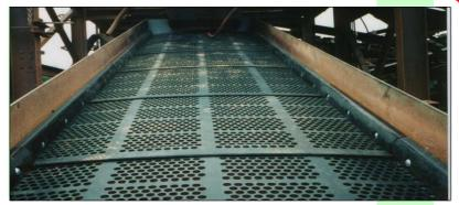
Rubbertend tensioned screen panels are a fabric reinforced rubber screen cloth that provide a cost effective alternative to woven wire or punched steel plate.
