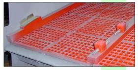
The self supporting modular panels are generally 315 and 305 in any length required . The most popular size is  $735/750 \times 315$ .
