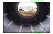
A full range of products for lining of washing and scrubber barrels. Lifter bars are moulded with an aluminium clamping rail which accepts industry standard drop forged "T" bolts.
