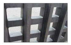
Perfect 60 rubber screen panels for primary screening. The panels are moulded with a fully self supporting frame and textile plies.
