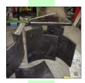
Steel backed rubber lining elements incorporate a highly abrasion resistant Perfect 60 compound moulded onto a mild steel backing plate. Ideal for a wide range of lining applications from sand and gravel of utes to dump truck liners. The DIN abrasion figure of 75 makes it one of abrasion resistant products on the market.
