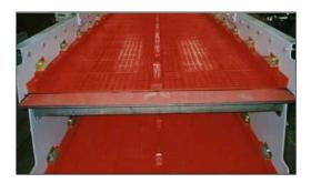
SCS Polyurethane modules are manufactured from very high grade, cut and wear resistant polyurethanes of various types.
