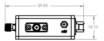
Dimensions are in (mm). Tolerances:  $\pm$  .015 mm
