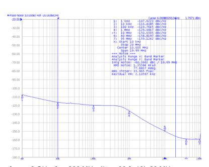
$f_{OUT}$  = 6 GHz,  $f_{PD}$ =200 MHz,Jitter=36 fs 12k-20 MHz
