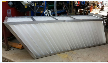
斜板連不銹鋼框架 Lamella Block with Stainless Steel Frame
