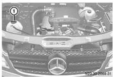
(1) Coolant expansion tank cap
