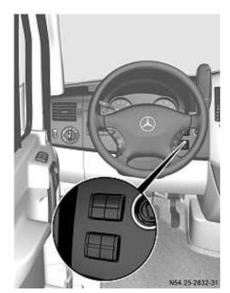
Switch unit between the steering wheel and ignition lock
