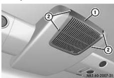
Air filter in the roof in the rear compartment
