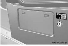
Vehicle identification plate with vehicle identification number
