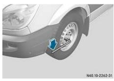
▶ Loosen the wheel nuts or wheel bolts on the wheel to be changed by about one turn
