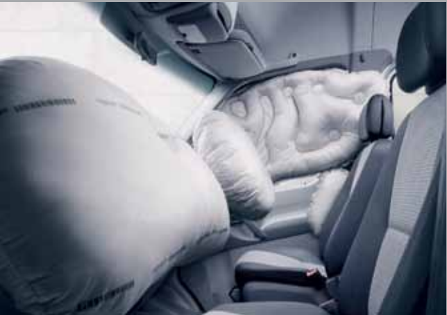
Air bags – optional window and even thorax bags can provide additional safety to driver and front-seat passenger airbags (shown activated for illustrative purposes only).
