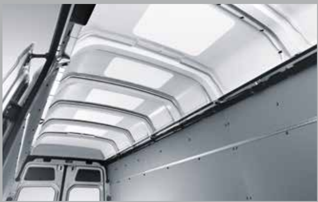
Super-high roof. Translucent sections in the roof shell of the super-high roof version improve lighting conditions in the load compartment.
