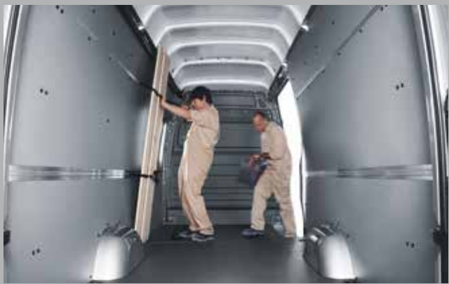
Flexible load-securing and cargo-retention system. Optional lashing rails in the floor, sidewalls and roof frame as well as tensioning straps for the lashing rails are available to secure loads.
