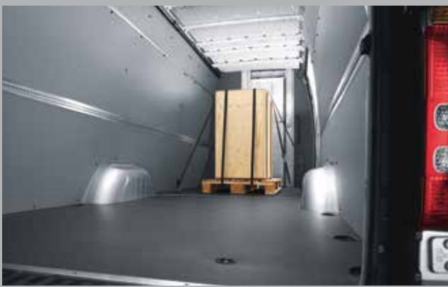
Cargo volume. A fourth body length and the optional super-high roof mean that up to 17 m³ of cargo space are available.
