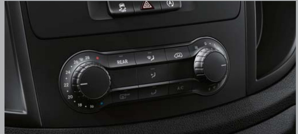
TEMPMATIC automatic temperature control regulates the desired temperature for the driver and front passenger.
