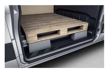
The pallet support in the step of the sliding door stabilises loads in the door area and is particularly useful when transporting Europallets or crates.
