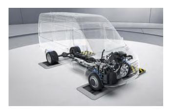
Front-wheel, rear-wheel or all-wheel drive<sup>1</sup> – the 3 drive variants for the Sprinter have virtually every transport task and every usage profile covered.
