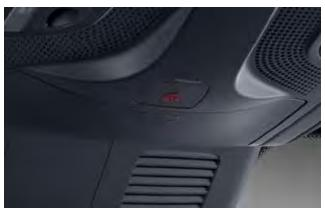
In the event of an accident, the Mercedes-Benz emergency call system sends out an emergency call automatically, which can help to speed up the arrival of rescue services at the scene of the accident substantially.
