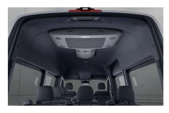
The high-performance overhead air conditioning system supplements the air conditioning in the front with an additional 11 kW of cooling output to deliver the ultimate in climate comfort in the passenger compartment.
