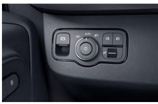
The electric parking brake is simply and conveniently operated via a button, avoiding the need to raise and lower a handbrake lever.
