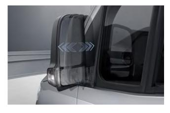
The electrically folding exterior mirrors are better protected against damage when folded and when space is tight in entrances and exits.
