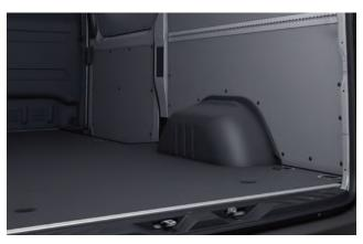
The even surface of the weight-optimised plastic floor facilitates use and maintenance of the load compartment and offers weight savings in the order of 18.5 kg in comparison to the standard wooden floor.<sup>2</sup>
