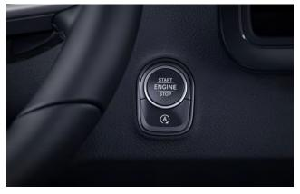
Starting the engine at the push of a button: the KEYLESS START drive authorisation system allows the engine to be started simply by pressing the start/stop button in the ignition lock. Please note: Vehicle locking and unlocking is still controlled by the driver.
