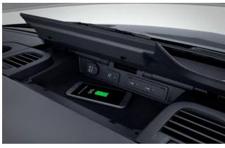
A wireless charging system provides simple charging of mobile devices which supports Qi standard 1.2 in the upper tray in the middle of the centre console.
