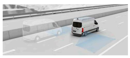
Blind Spot Assist with Rear Cross Traffic Alert can output visual and audible warnings to help prevent accidents during lane changing, when reversing out of parking spaces and when exiting from the vehicle.
