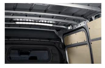
The two LED light strips under the roof illuminate the load compartment, for improved visibility inside when loading and unloading the vehicle.
