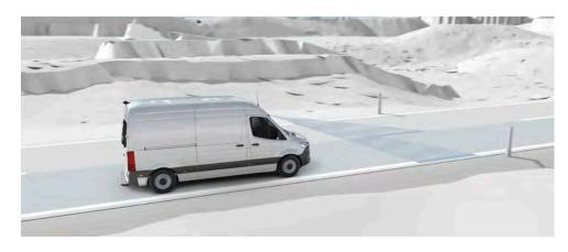
Active Lane Keeping Assist can help to detect when the vehicle is unintentionally leaving its lane, warn the driver and, if necessary, actively help to return the vehicle to its lane by means of braking intervention.
