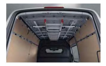
Internally fitted roof racks are available thereby protecting items against theft and preventing the need for external racking to be mounted.\!
