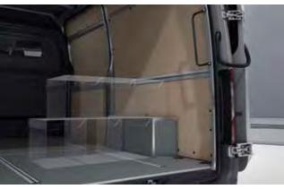
The wood trim on the wheel arches facilitates loading of the load compartment and protects the metal panelling from damage.
