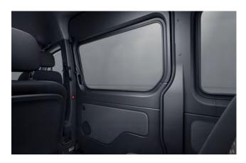
The sliding door with full plastic panelling on the inside enhances the appearance of the passenger or load compartment.
