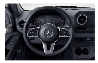
The multifunction steering wheel offers a convenient means of operating the on-board computer, vehicle functions and the multimedia systems and cruise control via touch control or steering wheel buttons, without the driver having to remove their hands from the wheel.
