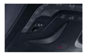
Swift breakdown assistance at the push of a button: Breakdown Management establishes a voice connection to the Customer Assistance Center (CAC) and enables assistance.
