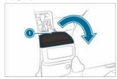
▶ Pull release catch (1) and lift the cover of the armrest upwards.
