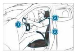
Observe the following when adjusting steering wheel (1), seat belt (2) and driver's seat (3):
