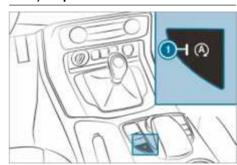
▶ Press the <a>A</a> button. If the indicator lamp (1) in the button is lit, the ECO start/stop function is activated.
