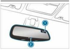
Current direction of travel ① is displayed in the rear-view mirror.
