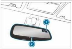
If the compass is not calibrated or is malfunctioning due to external influences, the current direction of travel is not displayed in the rear-view mirror. The display (1) then shows C.
