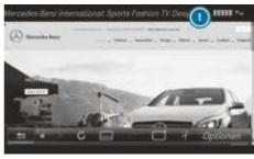
① Display of existing connection and signal strength of the communication module or the connected Bluetooth<sup>®</sup> device
