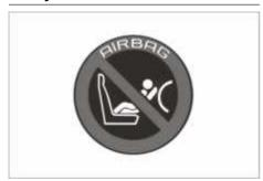
Vehicles without automatic front-passenger front airbag deactivation system have a special sticker on the front-passenger side of the dashboard which is visible when the frontpassenger door is open.
