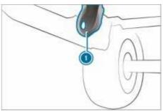
The rear towing eye ① is located under the bumper on the left side of the vehicle.
