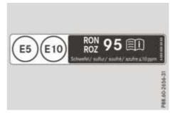
If the available fuel is not sufficiently low in sulphur, this can produce unpleasant odours.
