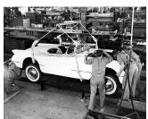
!Its radical fiberglass body was the only really new component on the 1953 Corvette. Everything else was directly off the Chevrolet parts shelf. Because of this, the first Corvette was essentially a regular 1952 Chevrolet
