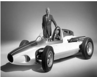
The idea of a [mid-engined Corvette](#) is not new. In fact, it was 60 years ago this year when the first functioning prototype based on that very idea was put together. Known as 1959 CERV I (Chevrolet Engineering Research Vehicle), this open-wheel single-seater rocket was the brainchild of Zora Arkus-Duntov, a Belgian engineer of Russian descent who joined [Chevrolet](#) in 1953, just after the birth of the first Corvette.
