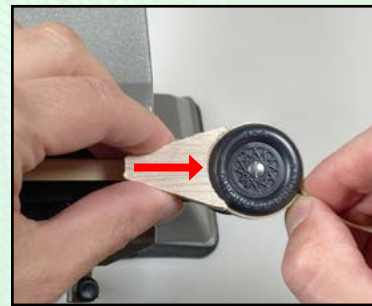
Place the fender on the car and hold in place while pushing against the wheel.
