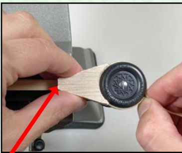
Test fit the fender and mark its edge on the body.
