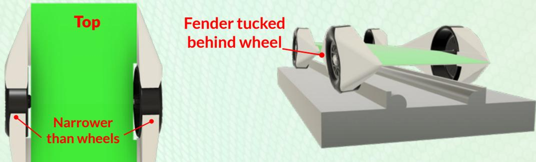
Failure to properly shape the fenders will **result in a significant increase in drag/friction**, negating the benefit of the fenders. In many cases, a poorly done fender car will be **SLOWER** than a similar car with no fenders.
