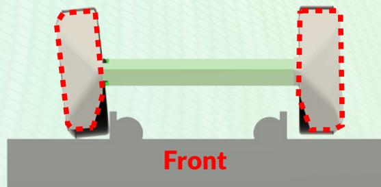
3. Trailing Edge - Great care should be taken when shaping the trailing edge fenders; they need to be more narrow than the wheels, tucking in behind the front wheels to ensure that **no part can stick out past the wheel**.
