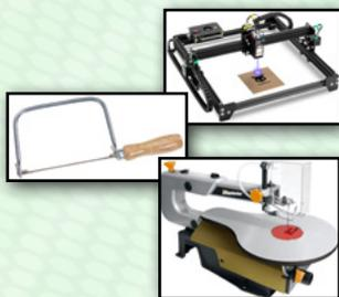
These bodies are built using a coping saw by hand, a scroll saw, or a CNC router/laser. For hand cutting, the design is sketched onto the wood block. A hole is drilled through the block that allows the saw blade to pass through so the builder can cut the interior features of the body. A top needs to be added (glued) to the car. League racers prefer 1/64-inch thick plywood for this purpose.
