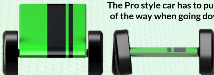
The Pro style car has to push less air out of the way when going down the track.
