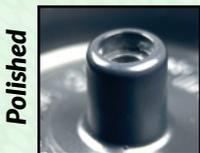
Inspect the tread edge and inner hub, ensuring the surfaces are smooth with no remaining flashing/burs and the plastic is shiny. A magnifying glass or [jeweler's loupe](#) is a handy tool for wheel inspection.
