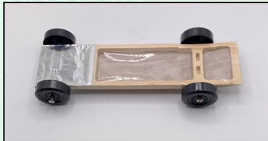
Insert the wheels and axles all the way. For rail riding setups, you will want the right front axle head of the bent axle to point downward.
