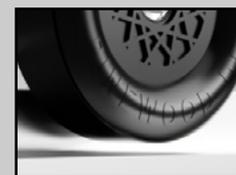
**If running a rail riding setup with a raised front wheel, you do not need to polish and wax all of the surfaces of the raised wheel. Instead, prepare only the tread and tread edge.**
