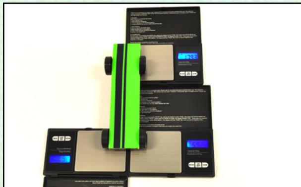
Weight is moved around the body to arrive at the target weight distribution for each wheel. The racer's goal is to find the amount of weight on the front wheel that results in a stable car and maximizes potential energy.
