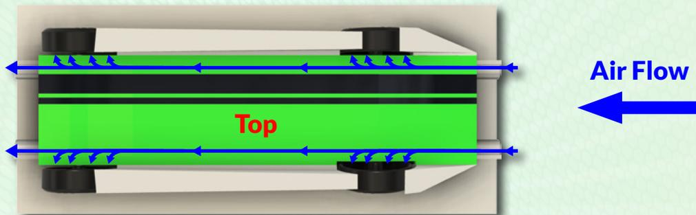
Air redirected by the wheels or fenders can flow into the rear cavity or inside of the wheels. This airflow creates drag and turbulence. However, there is a solution to keep air out of the wheel cavities known as air shields available [here](#).
