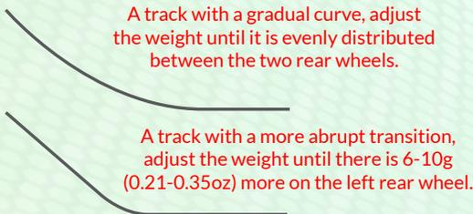
Once the correct weight distribution is determined, the weights can be affixed to the car using double-sided tape and covered with foil tape.
