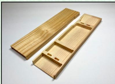
These car bodies are built using a hand router or CNC router to cut out pockets on the bottom of the car for the weights and remove unneeded material from the body. These bodies tend to be .3125 to .375 inches thick.
