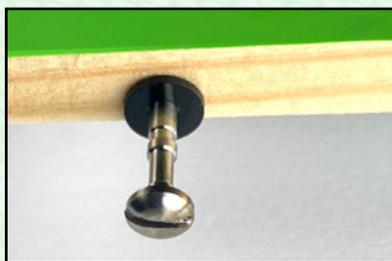
In the professional leagues, racers will use washers made from Delrin™ or Teflon™ glued to the body to reduce friction. However, washers are prohibited in most Scout races.
