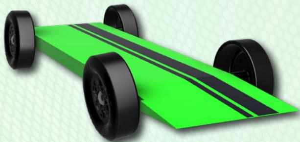
The often repeated mantra among league racers regarding the car body is **“Thin to Win!”** In other words, a thin body is the fastest. As a Pinewood Derby® car speeds down the track, it has to move the air it encounters out of the way. This **pushing of the air creates drag** and slows the car. Therefore, with all other things being equal, a car with the smallest area pushing against the air will be the fastest.
