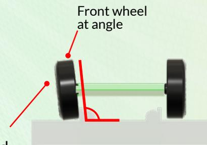
When the front of the car is higher than the rear, it causes a toe-out orientation on the rear wheels, increasing friction and allowing air to enter the back of the wheels, slowing the car.
