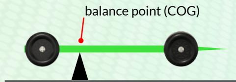
The balance point is measured as a given distance in front of the rear axles (i.e. 1 inch).
