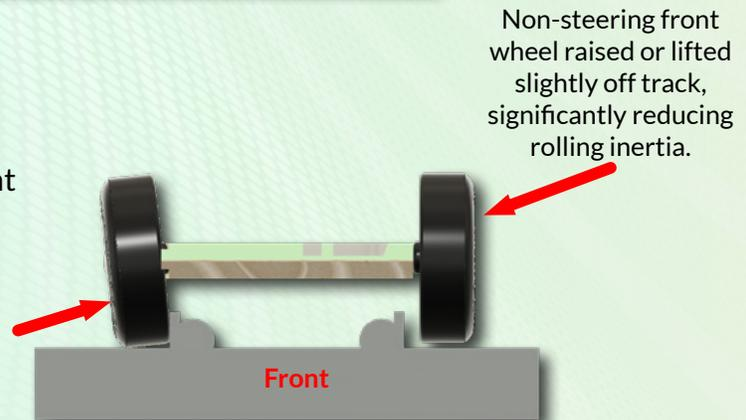
Non-steering front wheel raised or lifted slightly off track, significantly reducing rolling inertia.
