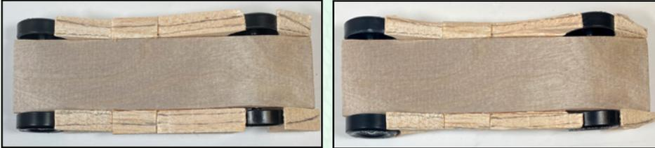
**STEP 3:** For the trailing edge fenders, cut in a bit more behind the front wheel than the front, leading edge fenders. You want to ensure that **NO PART** of the trailing fender can stick out past the wheel.
