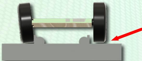
Non-steering front wheel raised or lifted slightly off track.
