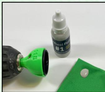
**STEP 2:** Apply a small amount of polish to the microfiber cloth (or use a cotton swab). Spin the wheel, using light pressure, polish the tread edge with the microfiber/polish for 1-2 minutes. Use a wet paper towel, cotton cloth, or soft bristle toothbrush to clean any remaining polish on the wheel. **STOP BE CAREFUL with the cloth near the**
