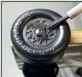
way under the axle head and into the wheel bore. Turn the car so the wheel faces the ground and spin the wheel several times. Repeat this process with the inner hub. Apply graphite and tap the wheel to spread the graphite into the inner hub and between the wheel and the car body. Turn the car so the wheel faces up and spin it several times. A soft bristle paintbrush works well to push graphite under the axle head and onto the inner hub. Add more graphite and repeat.
