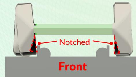
These notches ensure the wheels touch the rails and the fenders do not.
