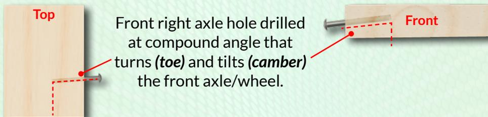
**Some race rules prohibit the bending of axles. If running a rail rider setup, drilling the hole at the compound angle to induce steer is the only option.**
