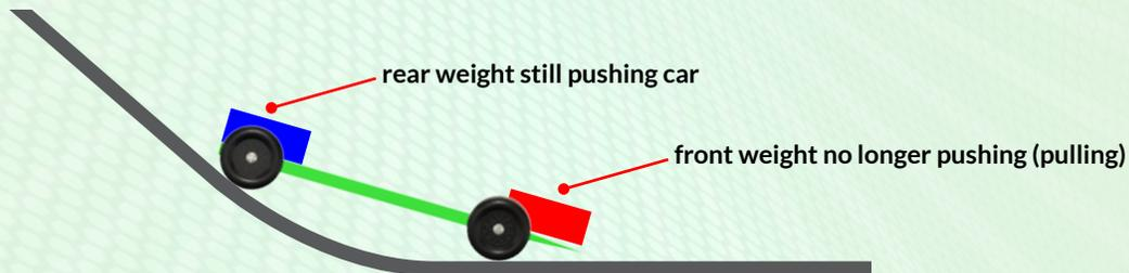
Notice the **rear weight** is still on the hill and falling, pushing the car. The **front weight** on the flat part of the track is no longer falling, therefore no longer pushing (or, in this case, pulling) the car. The extra push made by the **rear weight** significantly affects the car's speed once it is on the flat portion of the track (see video)! →
