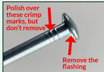
Removing the crimp marks on the axle shaft will significantly reduce the diameter of the axle. Crimp mark removal gives the wheel more room to move on the axle, making it more likely the wheel will vibrate, causing the car to wiggle. An unstable, wiggling car is slow.
