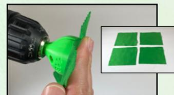
Cutting the cloth in fourths can help keep it from becoming entangled in the drill chuck!
