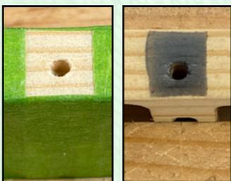
you will want to cover (masking or painter's tape) the painted area around the wood to keep graphite off other parts of the car. Make several graphite applications; you can't do too much.
