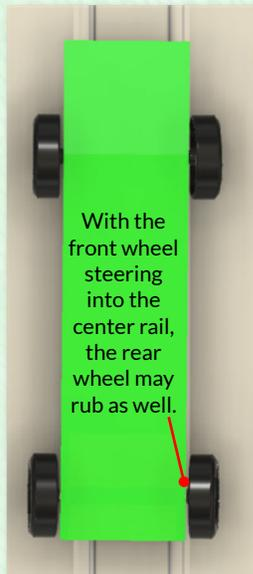
The front wheel steers into the rail to stabilize the car. A stable car is much faster than one that wiggles. However, if not addressed, the rear wheel on the same side as the steer wheel will also rub the center rail creating additional friction that yields no benefit.
