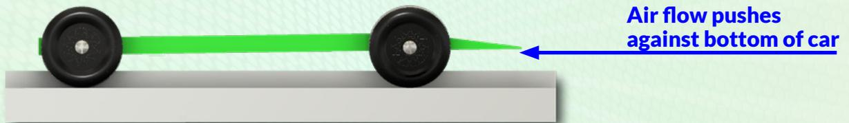
The front axle hole needs to be placed at a **precise amount higher** than the rear axle holes to eliminate the problem of the front of the car being higher than the rear. This placement ensures the rear wheels are not in a toe-in or toe-out position.
