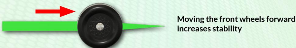
However, as with most facets of Pinewood Derby®, there is a **trade-off between speed and stability** regarding wheelbases. The shorter the wheelbase, the more potential there is for speed. However, the shorter wheelbase can also lead to instability, slowing the car.
