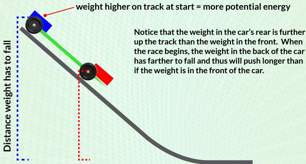
There is a point on the track where the car transitions from being on the hill to running on the flat part of the track.
