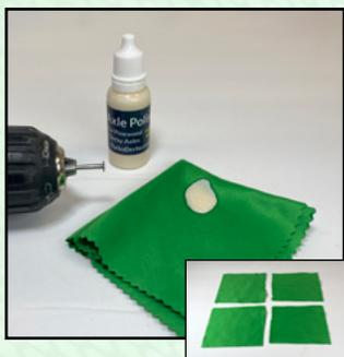
Wash the axles thoroughly with water, and wipe with a cloth or cotton towel. Then soak for 5-10 minutes in either isopropyl alcohol or ammonia-free glass cleaner. Inspect them under [magnification](#) to ensure there is no residue from the polishing process or lint on the axles. Be careful not to touch the axles' polished surfaces, wipe them again, and put them away in a clean, safe place.
