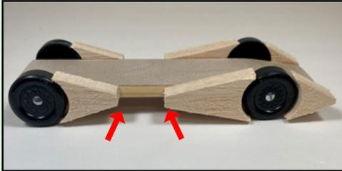
Can leave the center open and angle the fenders edges, sanding them flush to the body.
