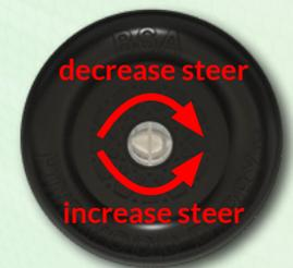
Setting steer is a balancing act between the amount of steer and the weight on the front wheel. If you have more weight on the front wheel, the car will need less steer; less weight will require more steer.
