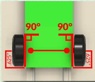
The rear wheels must be parallel to each other and the car body. Additionally, the wheels must be located directly across from one another. Finally, if rules do not prohibit, the rear axle holes should be placed 5/8ths (0.625) of an inch from the car's rear. Moving the rear wheels increases stability and maximizes speed by keeping the rear wheels on the hill of the track longer.
