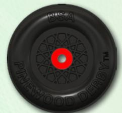
2. **Inner Hub:** Flip the wheel and repeat the above steps for the inner hub. If using a rail riding setup, burnish graphite onto the inner edge of the tread on the **front wheels only**. Burnishing graphite on the edge of the rear wheels will foul the actual tread and lead to an unstable car.
