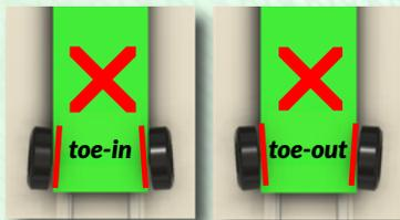
If the wheels are not parallel, they will be in a toe-in or toe-out orientation or a combination of these two. These orientations create a situation where the rear wheels are no longer in sync to steer in the same direction, increasing friction at the axle head and the contact point between the wheels and the track.
