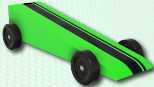
The wedge car is relatively easy to make; cut the block from the kit in half diagonally. This is accomplished using one of several types of hand saws (tooth saw, hacksaw, coping saw, etc.) or with power tools such as a bandsaw, jigsaw or scroll saw. Holes are drilled in the car's top, sides, or rear for weights.
