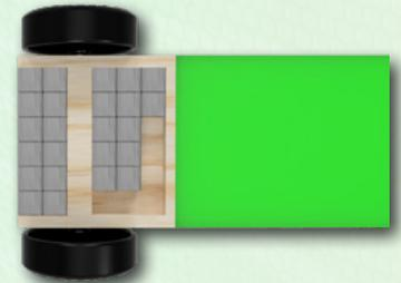
**Alignment** - The location and position of the axles in the car body are crucial to minimizing friction and therefore maximizing speed.
