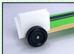
Four sheets of copy paper can be used to set the wheel gap.
