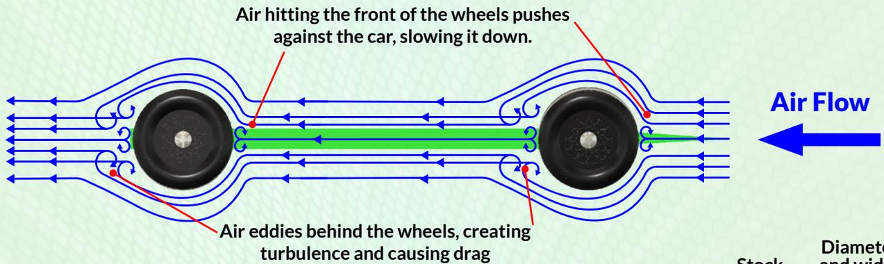
The wheels are a significant source of drag. They present a sizable forward profile and create turbulence (especially behind the wheel), further slowing the car. While the wheels can't be eliminated, if the rules don't prohibit it, they can be shortened (reduction in diameter) and narrowed (reduction in width), which decreases the amount of air they must move. Additionally, there are methods to move the air around the wheels more efficiently.
