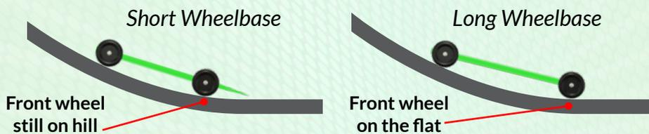
When determining a wheelbase for their car, the Race Team must consider the track condition they'll be racing on. For example, on a smooth aluminum track, a wheelbase of **4.75" offers a good balance between speed and stability**. For a rougher track where instability could be a concern, the Race Team might consider going with a 5.0" to 5.25" wheelbase.
