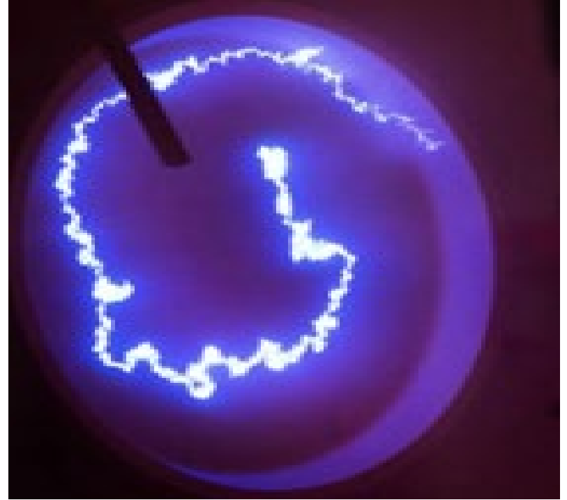
cathodic (vacuum) arc with magnetic field, as used in deposition of films and coatings
