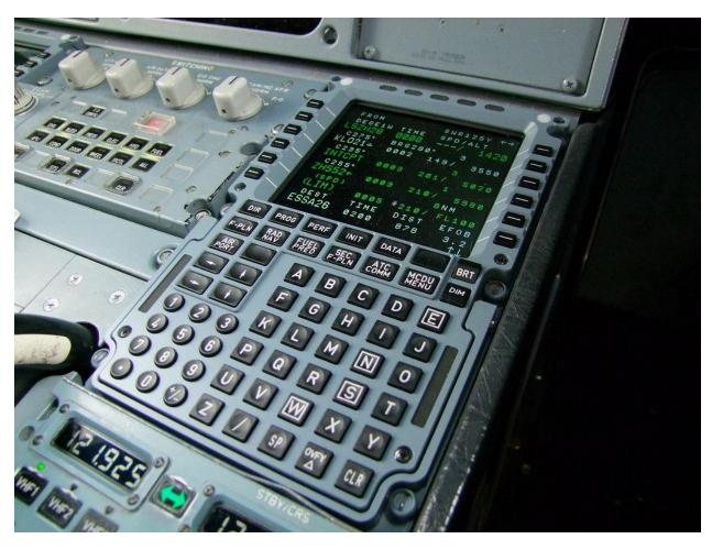
The FMS pulls in data from multiple sources to provide accurate information about the aircraft's speed, location, and ETA. The FMS uses
