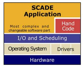
Figure 3.1: SCADE addresses the applicative part of software
