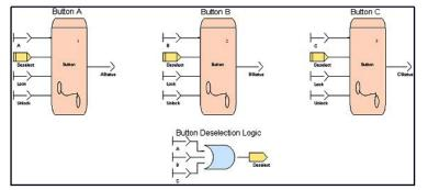
Figure 4.15: Three buttons in a parallel data flow
