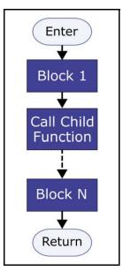
Figure D.2: Sequential structure of the generated code (without expansion)
