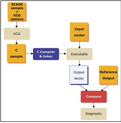
Figure D.5: Position of CVK items in the compiler verification process
