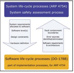
Figure 2.1: Relationship between ARP 4754 and DO-178B processes
