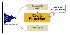
Figure 3.10: The cycle-based execution model of SCADE Suite
