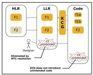
Figure 6.6: Elimination of unintended functions with MTC and KCG
