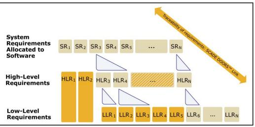
Figure 4.2: Development of high-level and low-level requirements with SCADE
