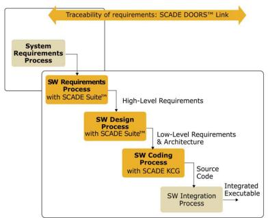
Figure 4.1: Software development processes with SCADE Suite
