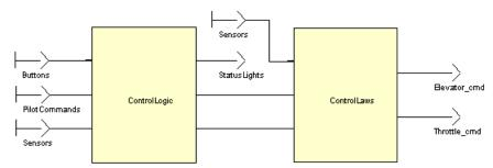
Figure 4.3: Top-level view of a simple flight control system
