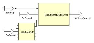
Figure 5.4: Connecting the observer node to the landing gear controller
