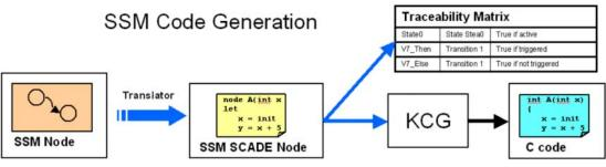
Figure 4.13: C code generation from SSMs
