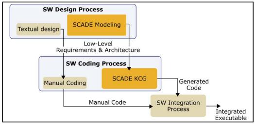
Figure 4.10: The software coding process with SCADE
