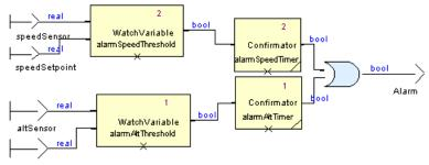
Figure 4.8: Alarm detection logic
