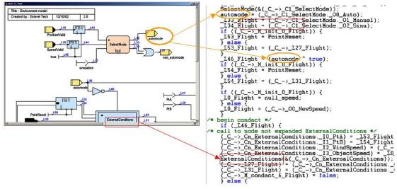
Figure 4.11: SCADE data flow to generated C source code traceability
