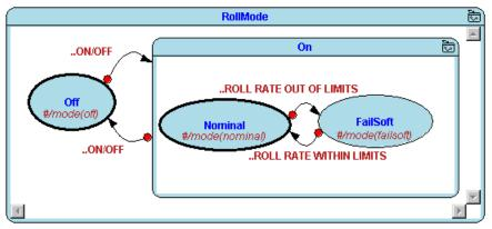
Figure 4.9: Safe State Machine for RollMode management
