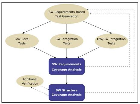
Figure 2.4: DO-178B testing processes
