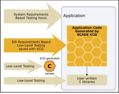
Figure 5.6: The combined testing process with KCG
