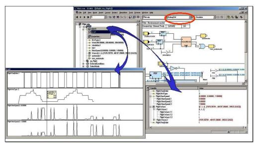
Figure 5.2: Simulation makes it possible to "play with the software specification"
