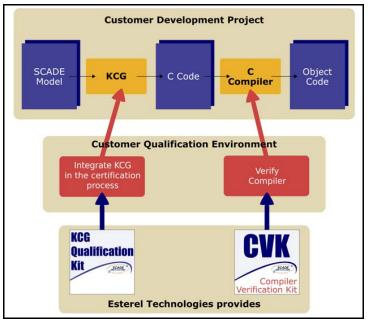
Figure D.1: Role of KCG and CVK in the qualification of the customer's development environment
