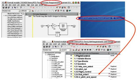
Figure 5.1: Traceability between SCADE LLR and HLR using DOORS<sup>™</sup> Link
