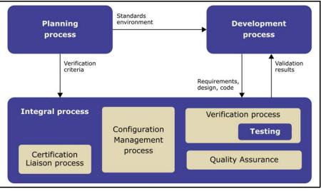
Figure 2.2: DO-178B life-cycle processes structure
