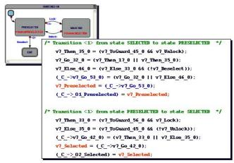
Figure 4.14: SCADE SSM to generated C source code traceability
