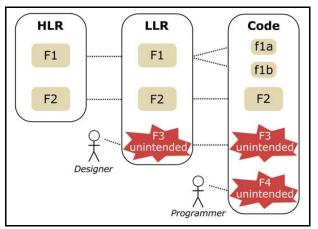
Figure 6.5: Sources of unintended functions in a traditional process
