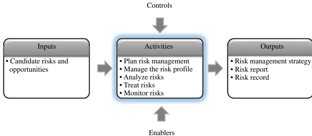
FIGURE 5.4 IPO diagram for the risk management process. INCOSE SEH original figure created by Shortell and Walden. Usage per the INCOSE Notices page. All other rights reserved.
