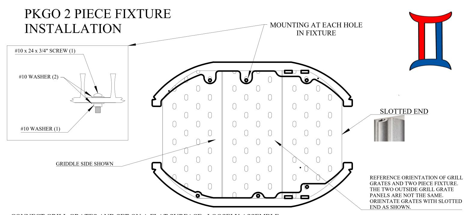
CONNECT GRILL GRATES AND SET ON A FLAT SURFACE. LOOSELY ASSEMBLE GRATES AND THE TWO FIXTURE PIECES WITH THE INCLUDED HARDWARE. SET ASSEMBLED PARTS INTO THE GRILL (GRATES UP), PUSH OUT THE FIXTURE PIECES TO SNUGGLY SET IN THE GRILL. TIGHTEN SCREWS WHILE THE ASSEMBLY IS IN THE GRILL. CAREFULLY REMOVE THE ASSEMBLY AND TIGHTEN ALL SCREWS. IT MAY BE NECESSARY TO REPEAT UNTIL DESIRED FIT IS OBTAINED.
