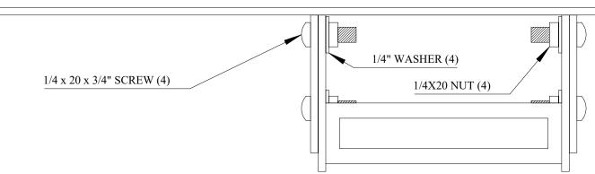
ATTACH LOWER BRACKET ASSEMBLY TO THE SHELF BRACKETS. LOWER ASSEMBLY WILL MOUNT INT BETWEEN THE SHELF BRACKETS USING THE SUPPLIED HARDWARE (SCREW, WASHER AND NUT PER HOLE)
