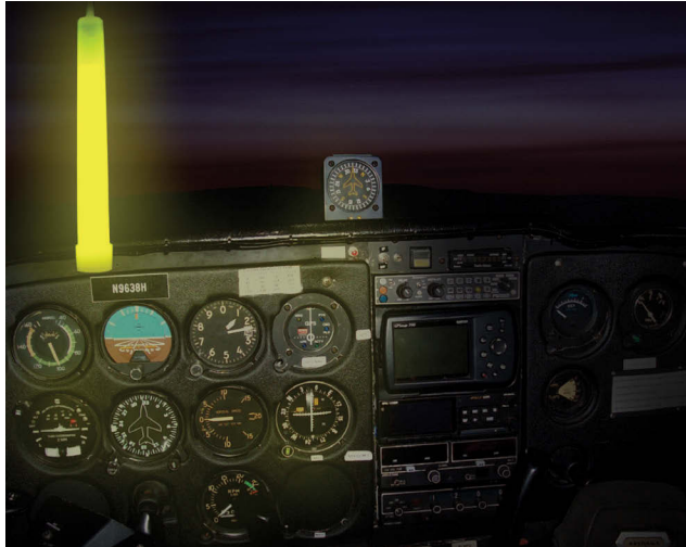
Figure 3-8. A chemical stick is useful to carry onboard the aircraft at night. It comes in various colors, intensities, and durations, and it provides ample illumination within the flight deck. This does not replace the regulatory requirement of carrying flashlights.
