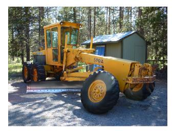
worthiness. The mechanical examination was that the motor needed to be replaced as coolant has been leaking into the crankcase and each cylinder was around half of needed compression output. Estimated repair and equipment costs could range up to \$70,000. Ownership of the grader also includes capital depreciation, maintenance, repairs, fuel, insurance, and an operator. The board is now in the process of making a decision as to whether the POA should remain in the heavy equipment business.
