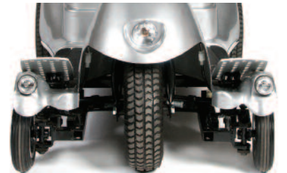
Quintell™ Self Centering Steering Defaults to straight travel with minimal effort
