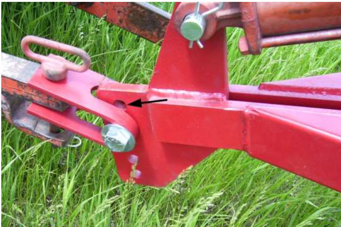
Figure 12: Changing Hitch Clevis on the Frame
