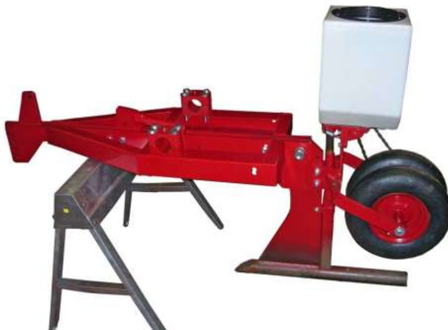
Figure 4: Frame and Seeder/Knife Assembly Mounted Together
