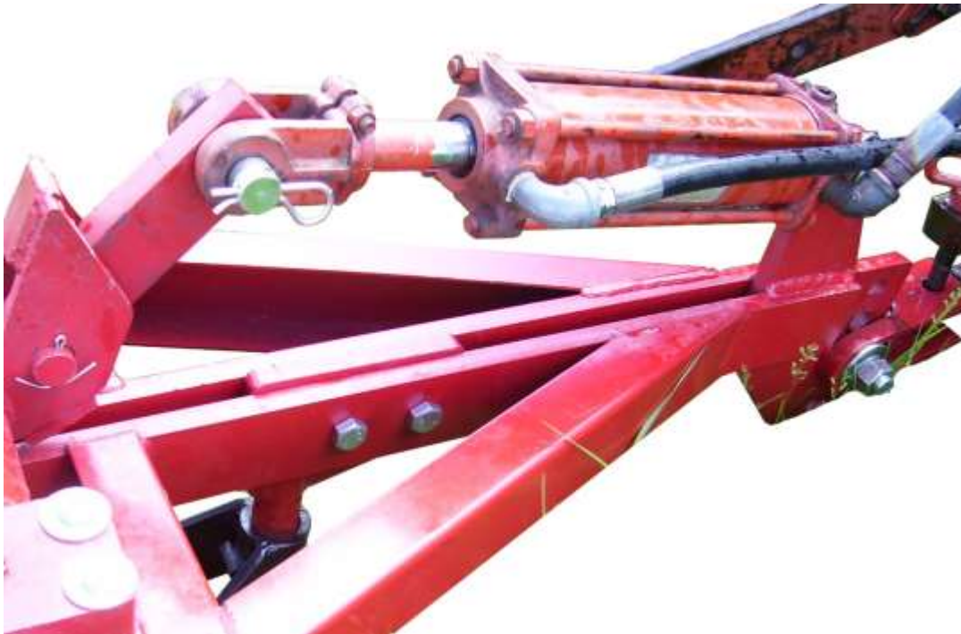
Figure 1: Typical 2" X 8" ASAE Standard Hydraulic Cylinder
