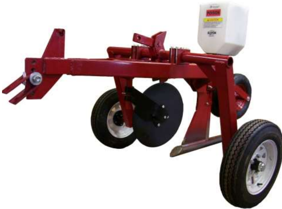
Figure 8: 18" Coultter Assembly as Installed
