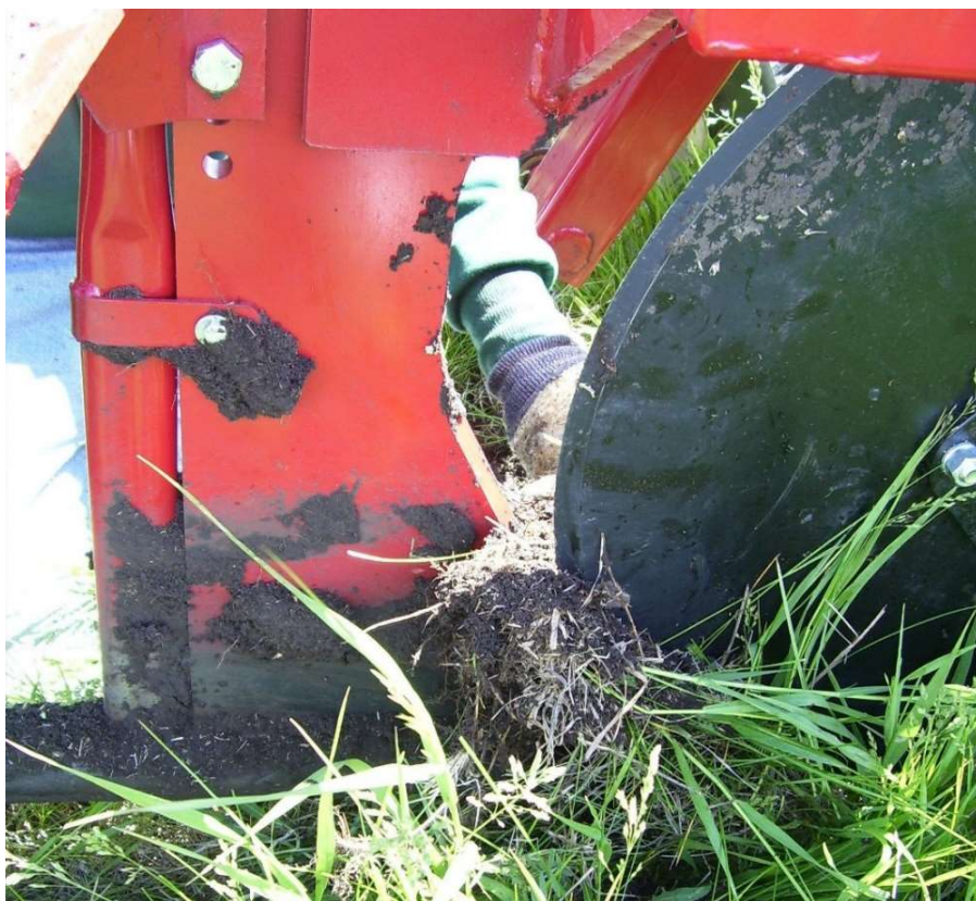
Figure 10: Roots catching on knife due to coulter blade set too shallow
