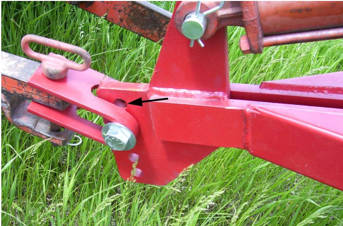
Figure 12: Changing Hitch Clevis on the Frame
