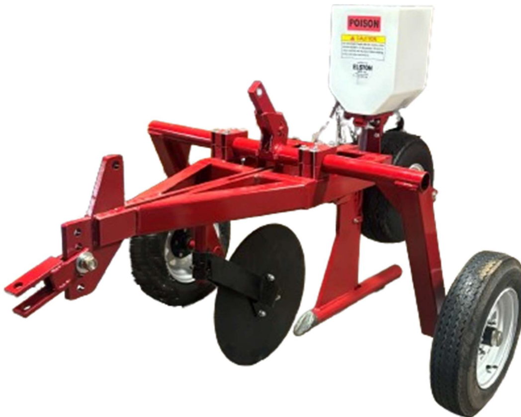
Figure 8: 18" Coultter Assembly as Installed
