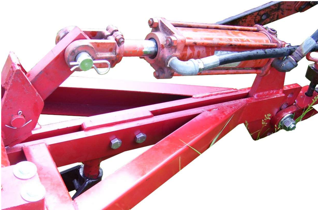
Figure 1: Typical 2" X 8" ASAE Standard Hydraulic Cylinder
