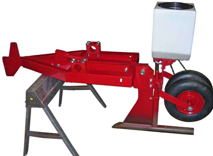
Figure 4: Frame and Seeder/Knife Assembly Mounted Together
