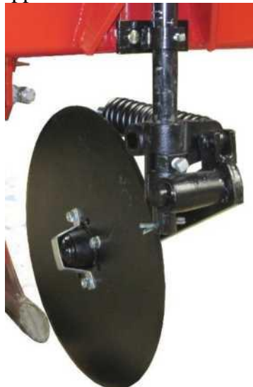
Figure 9: Completed Coultter Assembly
