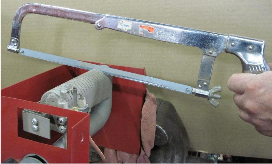
Figure 5 : Servicing burner slots with hacksaw blade
