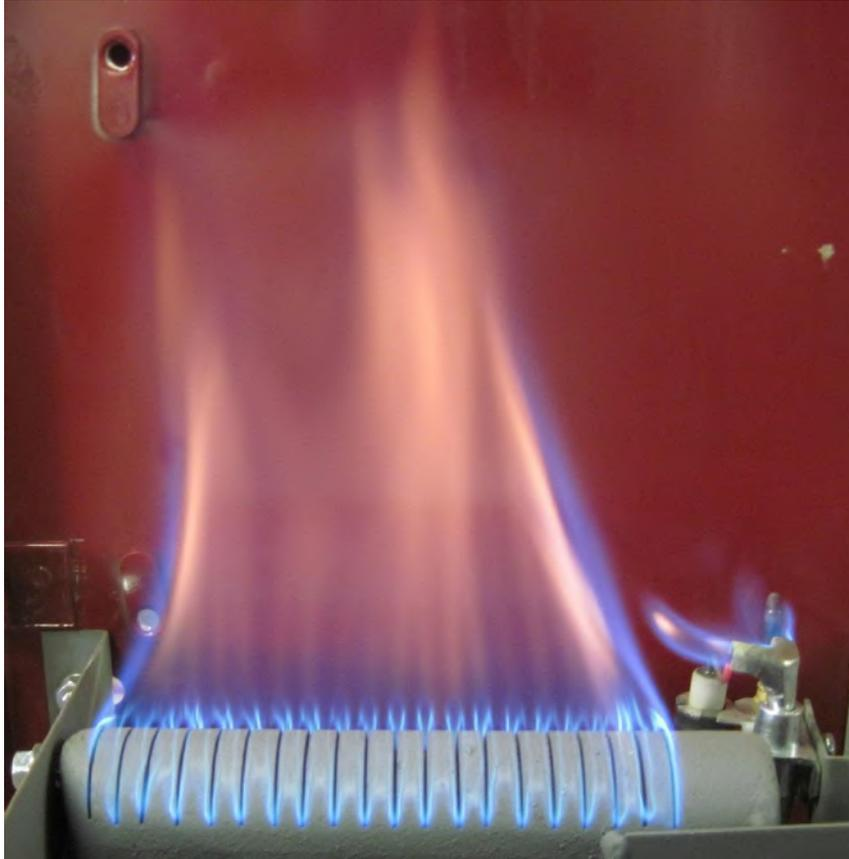
**Figure 8 : Burner with Insufficient Air**
