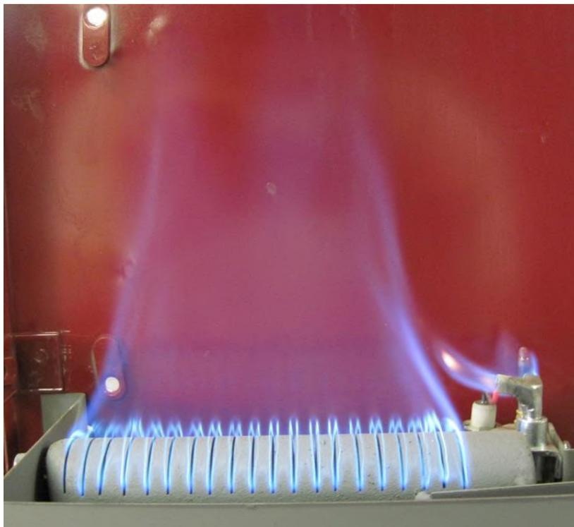
Figure 6 : Correctly Adjusted Burner Flame
