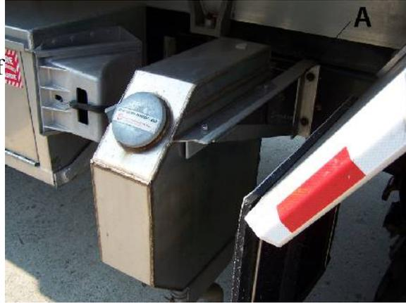
Once you have installed the sander tanks, you should trim the top of the grit discharge boots to provide 4" ground clearance when the bus is loaded. Mount the boots on the outlets on the aluminum operating unit with the included clamps. If necessary, we recommend rotating the boots on the outlets to center one in front of each tire.
