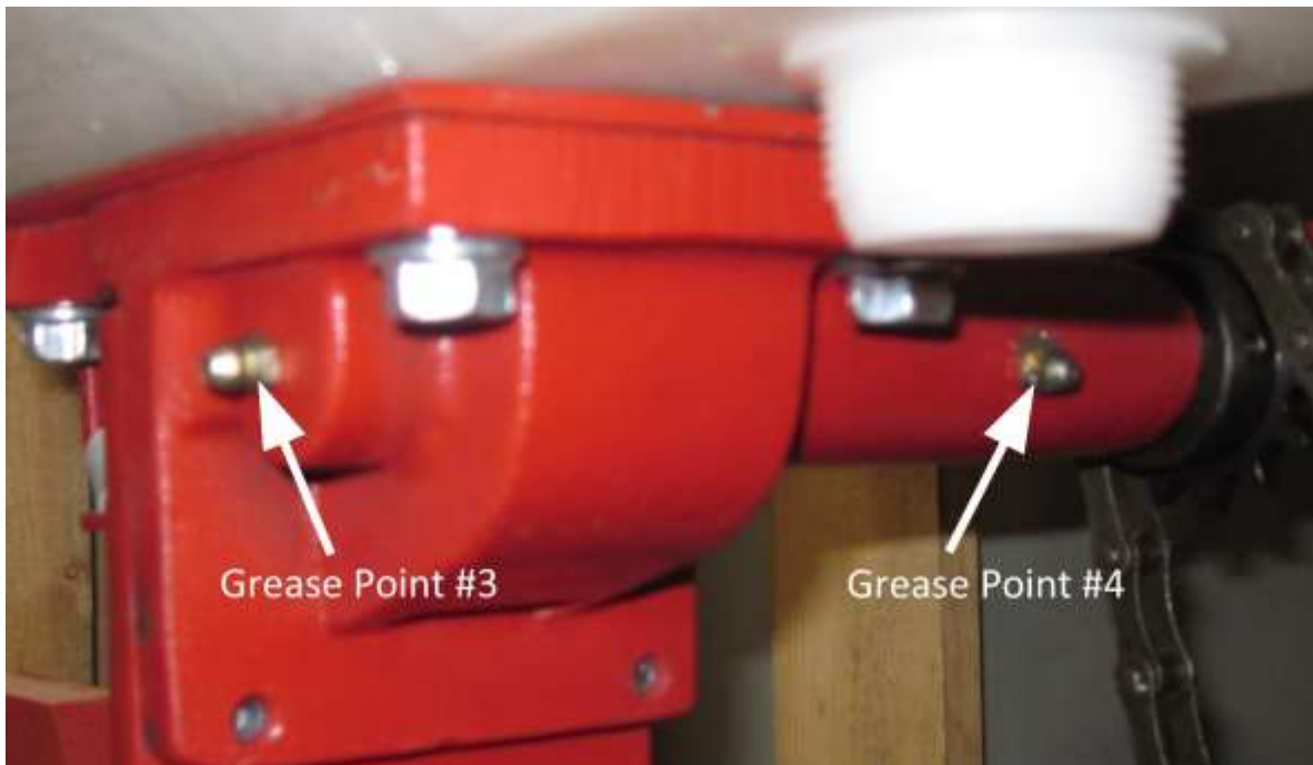
Figure 14: Grease points on GA-300 seeder casting
