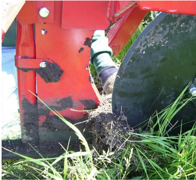
Figure 8: Roots catching on knife due to coulters blade set too shallow
