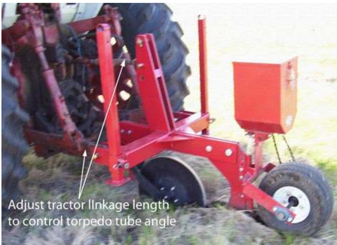
Figure 6: Adjustment of tractor link to control torpedo tube angle
