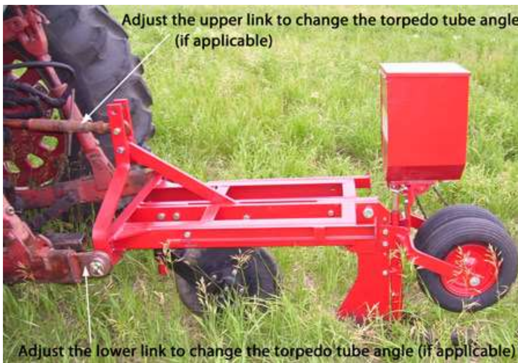
Figure 10: Adjustment of tractor link to control torpedo tube angle
