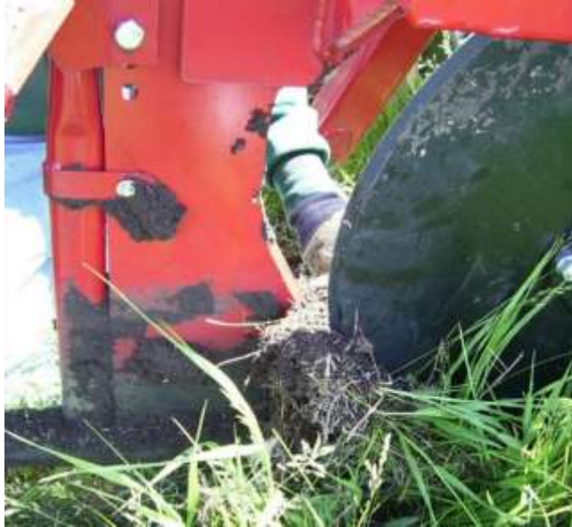
Figure 8: Roots catching on knife due to coulter blade set too shallow
