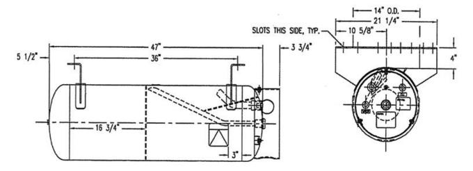
Figure 2: Dimensions of Tank
