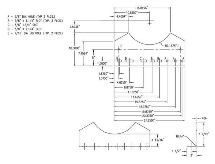
Figure 3: Bolt Hole Dimensions for Tank Bracket Shown in Figure 2
