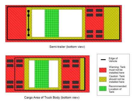
Figure 1: Installation Location of Tank
