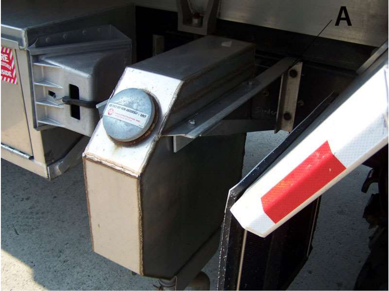
Figure 6: S-N861 Sander installed with custom angle brackets
