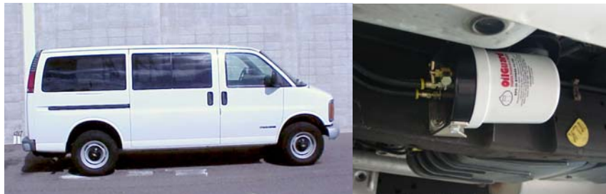
Figure 5. Chevy passenger van with bypass filter installed
