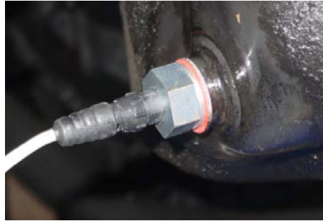
Figure 14. Oil sensor location at the bottom of oil pan
