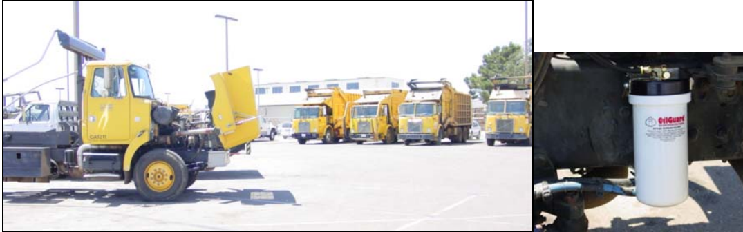
Figure 6. Diesel roll-off trucks and bypass filter
