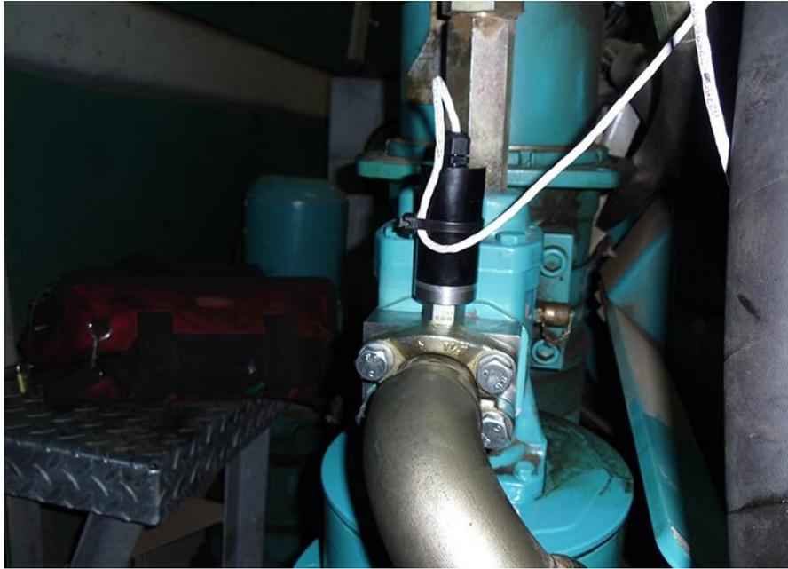
*The VSI sensor installed in the oil stream on the exit side of a wind turbine's oil filter.*
