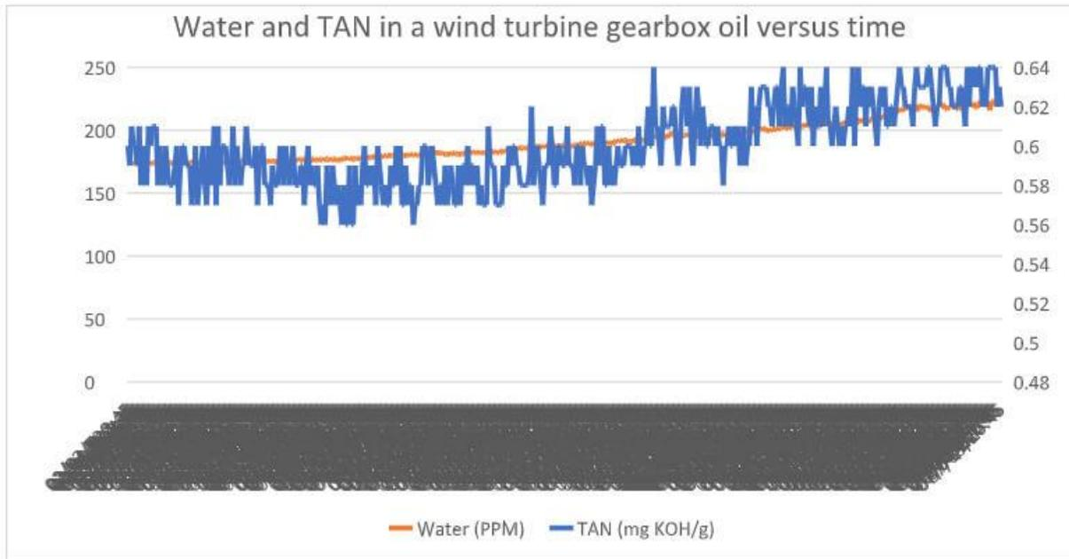
*The orange line plots the water content in the oil of a wind-turbine gearbox from February to July, on the left scale in parts per million. The blue plot tracks the Total Acid Number (TAN) on the right scale.*
