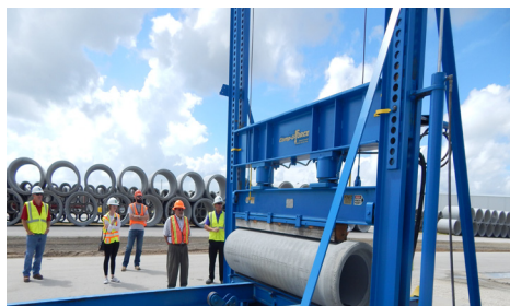
Three-Edge Bearing (3EB) Testing 18-inch Diameter Reinforced Concrete Pipe at County Materials in Astatula, Florida
