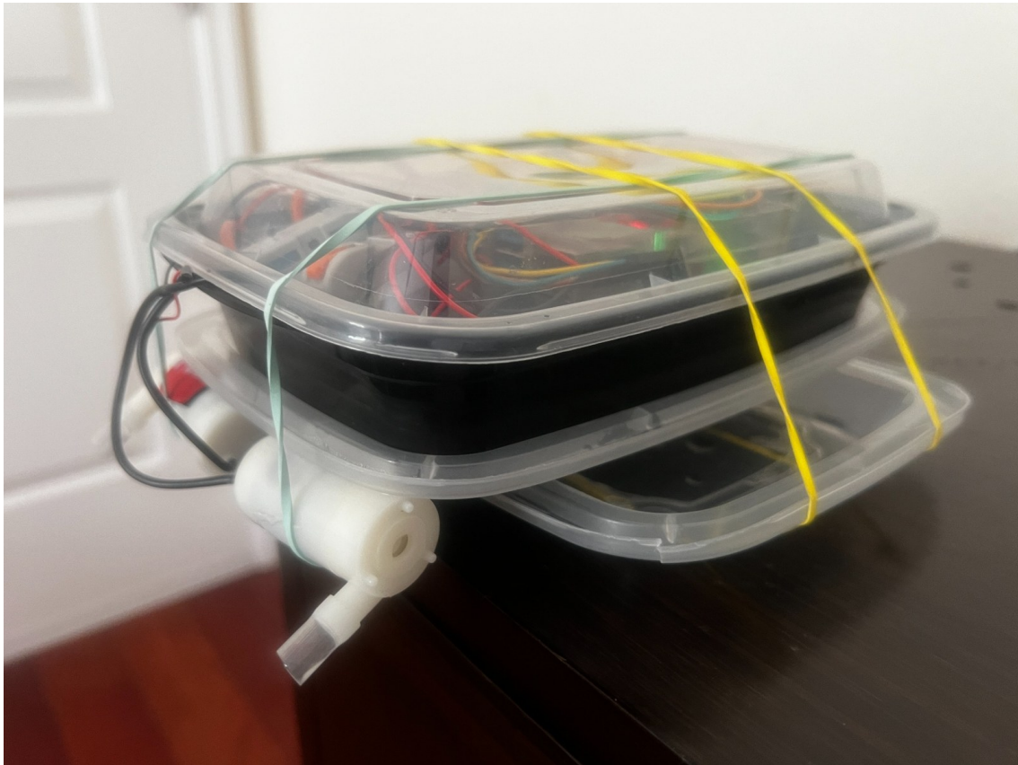
Figure A3. Layered under-plate/lid structure and laterally separated propulsion.
