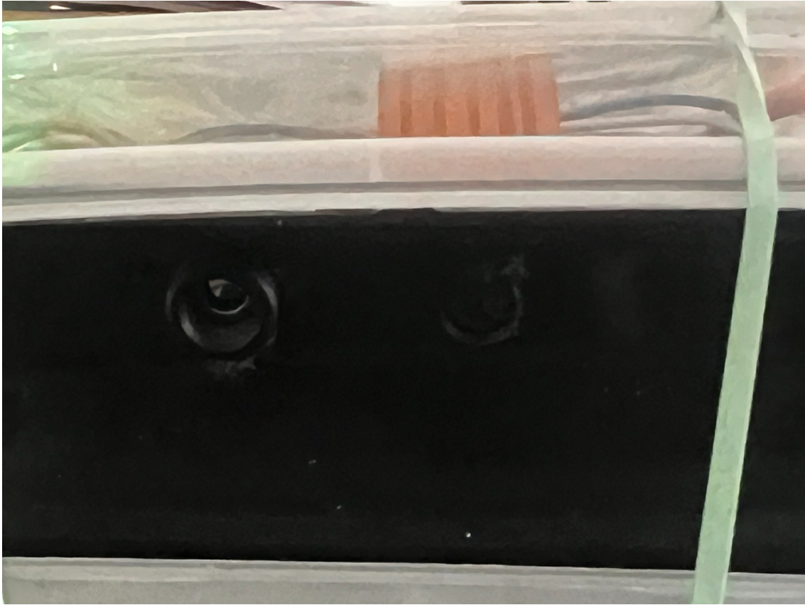
Figure A5. Forward sensor openings; preserve unobstructed RGB and thermal views.
