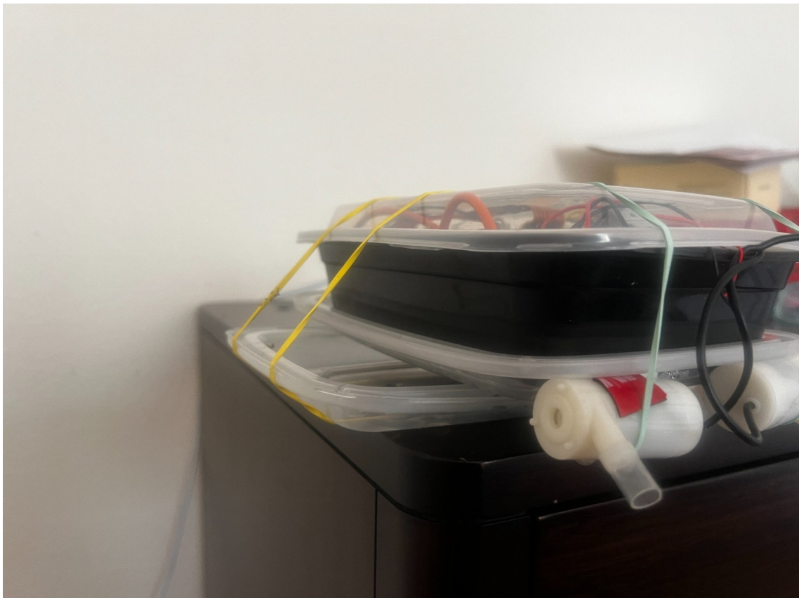
Figure A2. Oblique view showing the enclosure, transverse support and pump/tubing arrangement.
