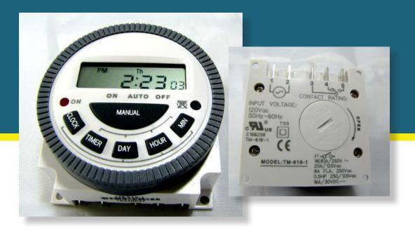
**The TM619 is a 7 day timer** that allows up to 8 on/off functions per day. It comes in 4 specific voltages: 12VDC, 24VAC/VDC, 120VAC and 240VAC. First, please check that you have the correct voltage for the application. The specified voltage is for the timer only. The output to your timed device goes through the contacts of the output relay which is rated to a maximum of 16a resistive and 8a inductive at 250VAC, 20 amps resistive at 125VAC and 16a at 30VDC.
