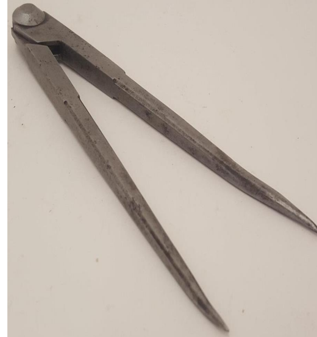
FIRM JOINT DIVIDER
