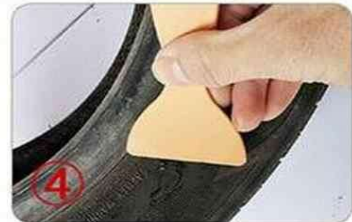
4 Press for a few minutes and leave for 24 h
