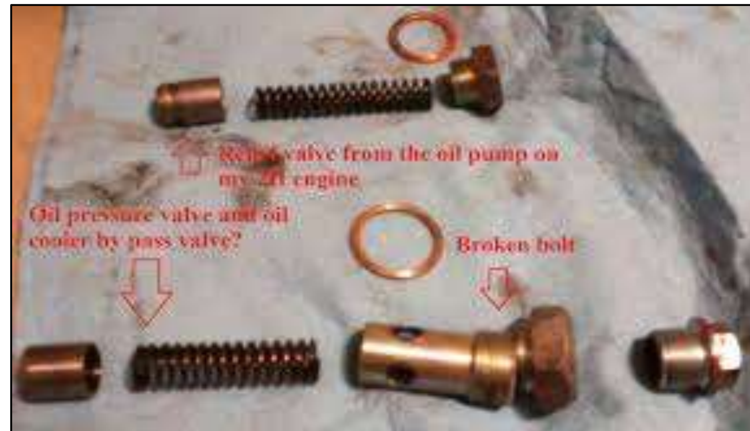
Failure Pressure relief valve
