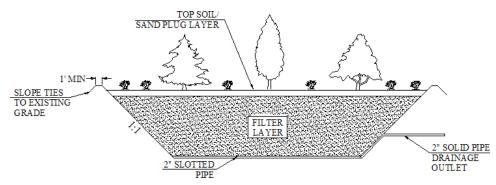
sit on the surface for a while because they have sand plugs or other design features on the top to catch the water. This allows the water to slowly enter the filtering layer, in this case a layer of fly ash and charcoal, at a proper pace; if it came through too quickly the filtering would not be effective. That's the basics. The cleaner water then empties through a drain, moving toward a creek, stream, or waterway if one is nearby.
