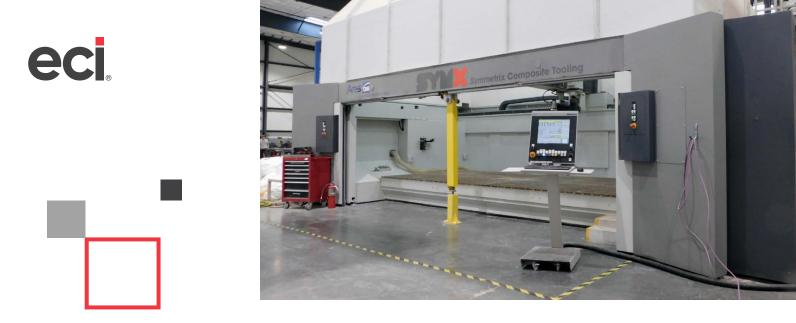
"At Symmetrix, we produce cost-effective, accurate tooling on schedule," John says. "We achieve sub-millimeter accuracy (+/- .020) through subtractive shaping methods in low-shrink materials that don't absorb moisture."
