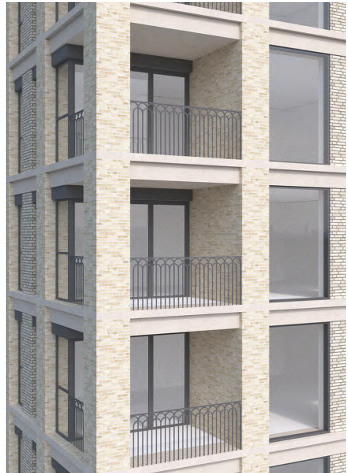
Balustrade detail to corner inset balcony
